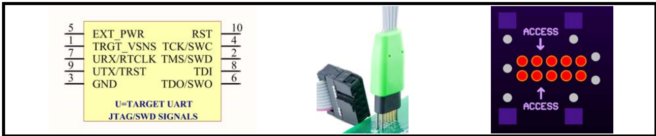
Figure 5: Engenuics/Tag Connect pin out, Tag Connect Cable, Example PCB Land Pattern Tag-Connect product photo from www.tag-connect.com/TC2050-IDC-NL
