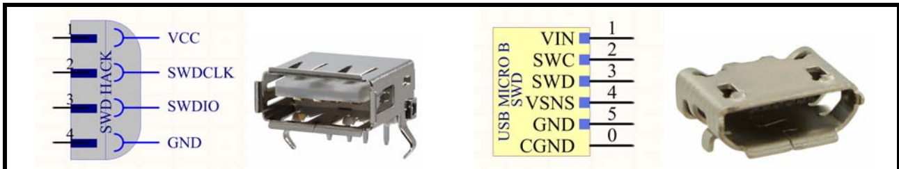
Figure 6: Programming adapter USB A (left) and target USB Micro B connector (right) Connector photos from www.digikey.ca
